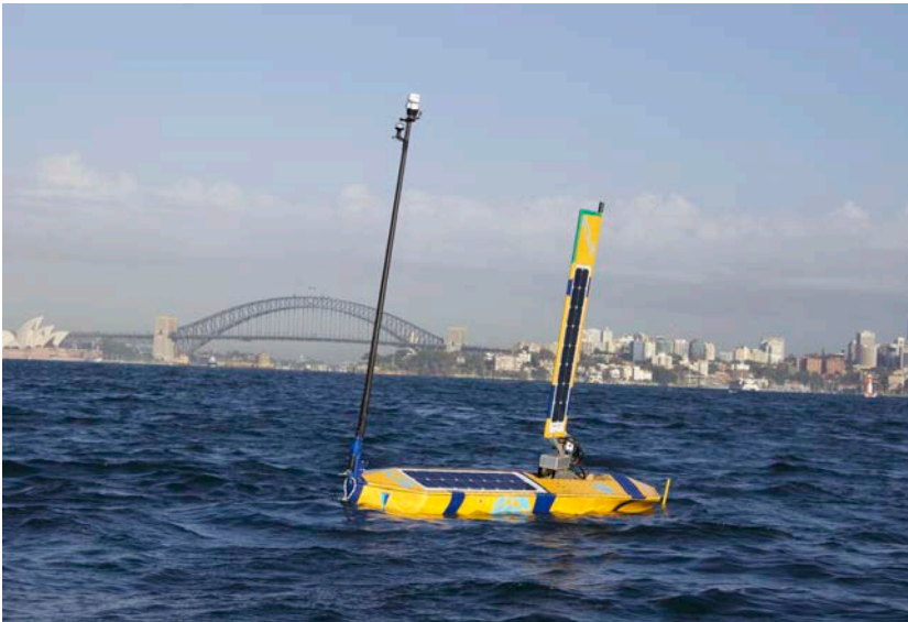
▲ Figure 2: Ocius 2.8m USV manoeuvring using wave & wind energy in moderate winds in Sydney Harbour.
