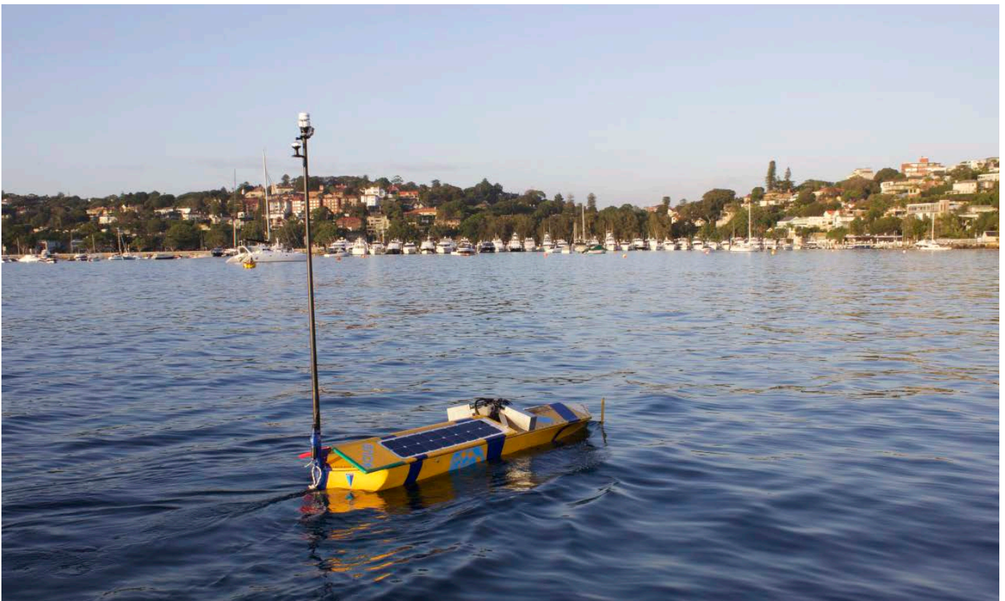
▲ Figure 3: Ocius USV self-deploying using active electric propeller power only.
